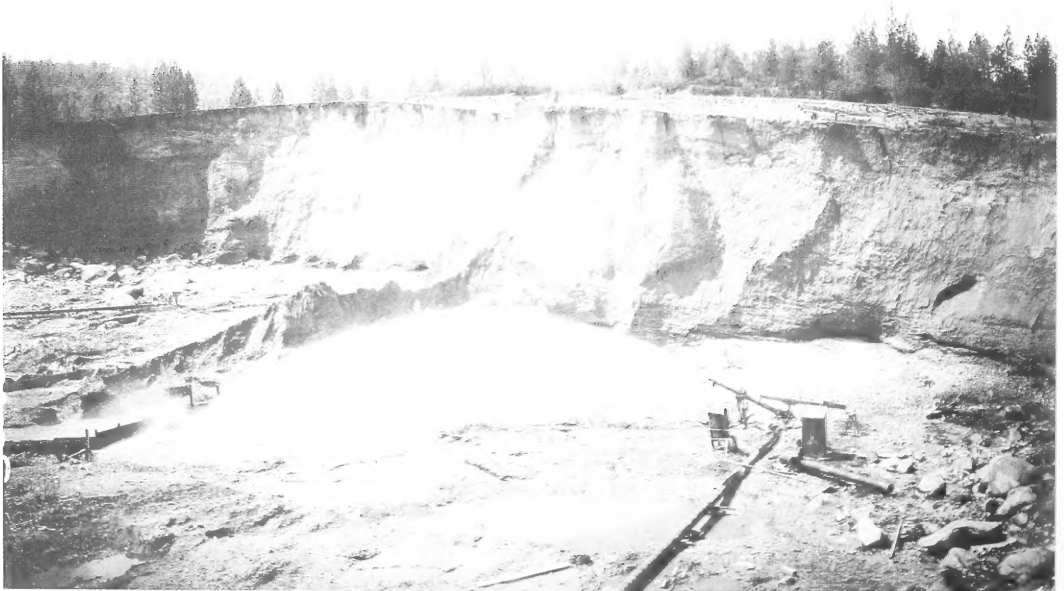
FIGURE 4. Hydraulic mining at the Esperance Mine, French Corral. Photograph by G.K. Gilbert. (G.K. Gilbert Collection [331.1.6.1; envelope #4], Alice Eastwood Archive, California Academy of Sciences Archives.)
